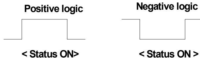
Figure 7.2 Positive and negative logic of general output signal
