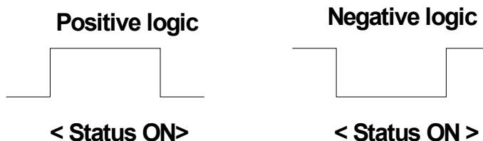
Figure 7.1 Positive and negative logic of general input signal
